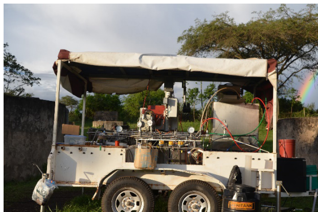
Fig. 2 Directly-coupled wind/solar submerged UF-NF/RO system for research on brackish water treatment
