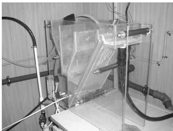
Fig. 5. Integrated membrane-electroflotation vessel.
