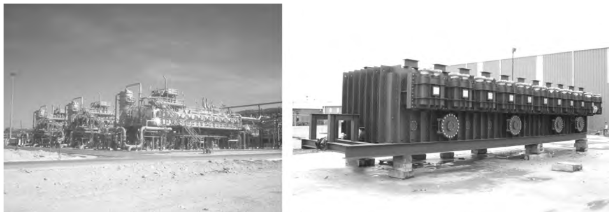
Fig. 3. MSF evaporators made of solid duplex stainless steel, 2205, for Melittah (left) and Skikda (Courtesy of Reggiane and Aquatech respectively).
