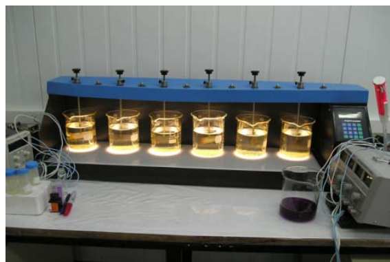
Fig. 1. Jar-test device used in the experiment.
