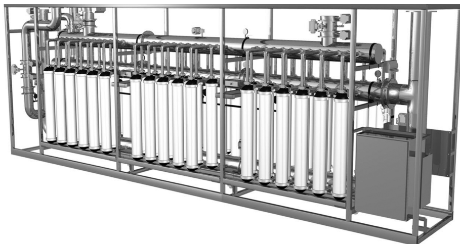
FIG. 8.22 Pressure driven capillary unit. Hydrablock with 66 (expandable to 72). Hydracap with UF modules. Filtrate capacity 29,000 m 3 /d (7.7 MGD).
