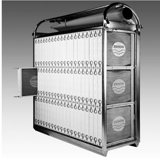
FIG. 8.16 Submersible capillary module assembly (Courtesy Zenon Corporation).
